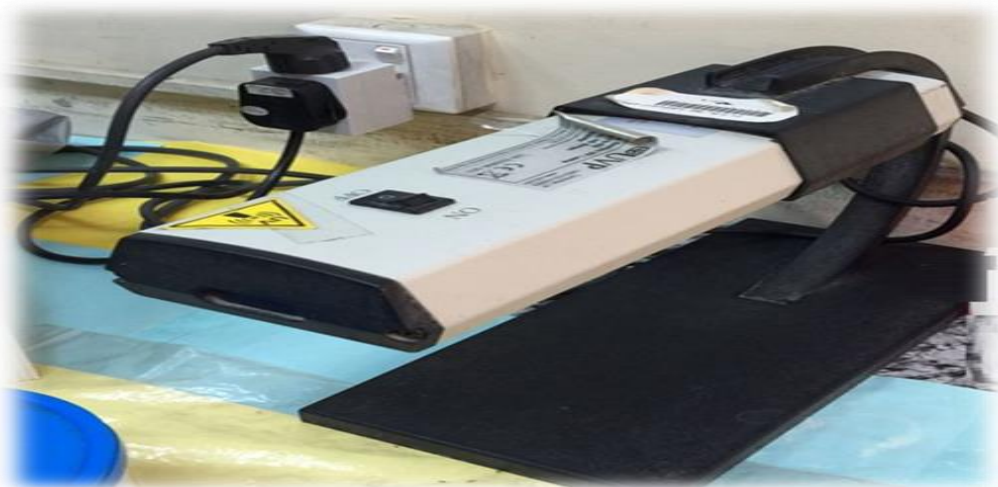
Figure (1): UVP Light Lamp 26-EL Series, Providing 365 nm wave Length
