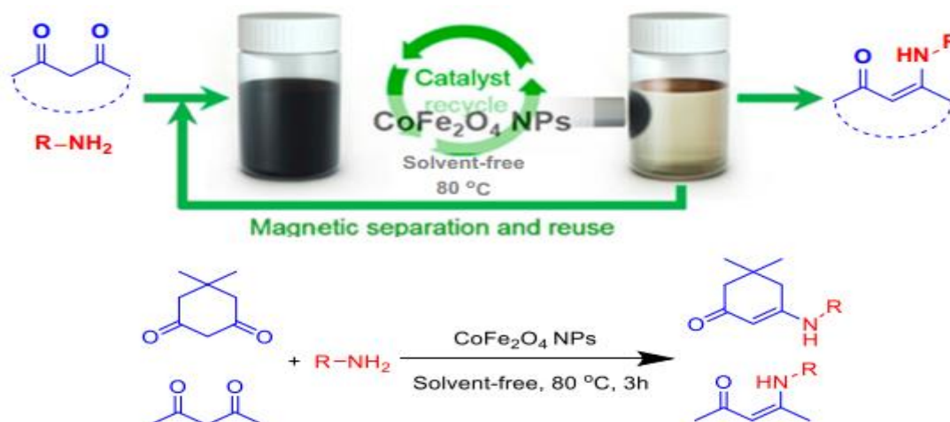
Scheme 20: Synthesis of β-enaminones catalyzed by \text{CoFe}_2\text{O}_4 NPs
